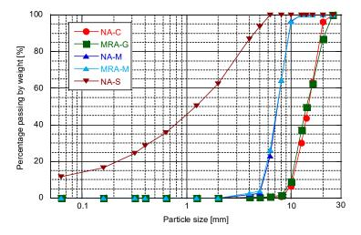
**Figure 1.** Aggregate particle size distribution. Note: NA-S: natural sand (0/6 mm); NA-M: natural medium gravel (6/12 mm); NA-C: natural coarse gravel (12/22 mm).
