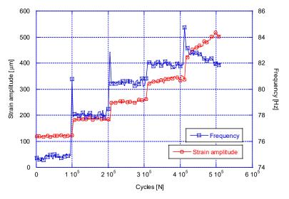
**Figure 10.** Comparison of the strain amplitude and the resonance frequency during a Locati fatigue test.
