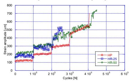
Figure 5. Strain amplitude evolution during a Locati test on the OPC mixes.
