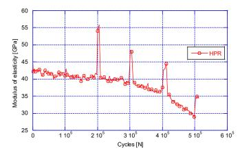
Figure 11. Modulus of elasticity evolution during a Locati test.
