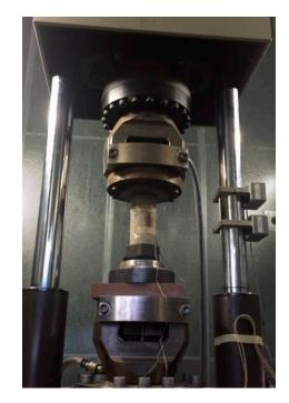
Figure 2. Zwick Amsler 400 HFP 5100 Vibrophore equipment. Schematic diagram of equipment and test specimen.
