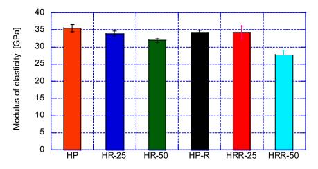
Figure 4. Modulus of elasticity of the different mixes.
