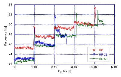
Figure 8. Resonance fatigue frequency evolution during a Locati test for OPC mixes.
