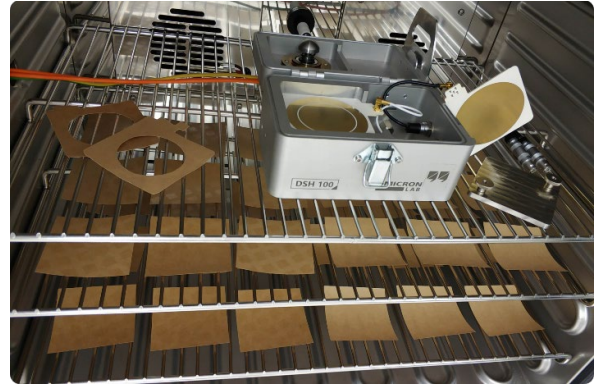
Fig. 1. Dielectric Material Analyzer with paper samples inside the climate chamber.
