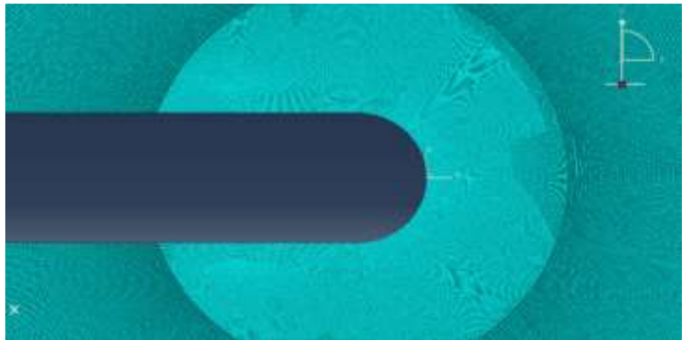
Figure 4. Mesh pattern in the vicinity of the U-notch tip.
