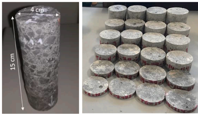
Fig. 4. Detail of a complete column of concrete plates (left) and a different series of plates (right).
