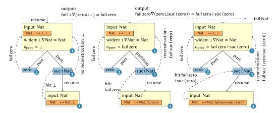
Fig. 4. Three iterations of a fixed point computation for input Nat. Iterations are separated by dotted arrows on top
