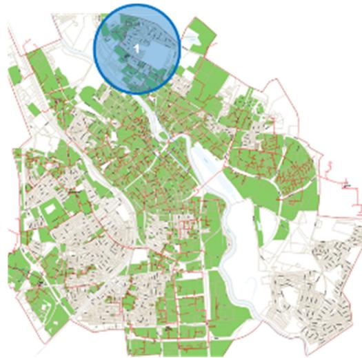
**Figure 1.** Tartu DH network (Estonia), with the demo area highlighted in blue.
