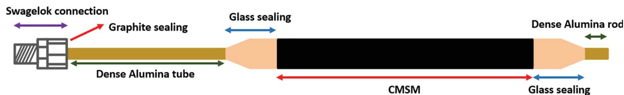
Fig. 1. schematic of a tubular supported CMSM with glass sealing on both sides.
