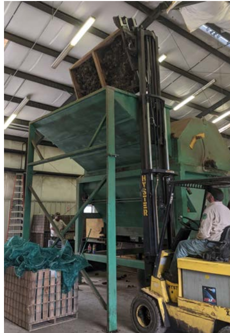
Allendale/Hampton/Jasper Sector Forestry Technician I Lowell Parnell dumps the dried cones into the extractor.
