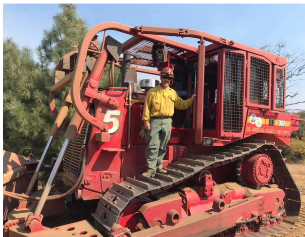
Holt with a LA County double-cab dozer that can seat two operators.
