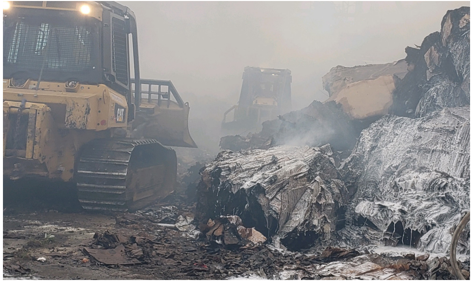
Lowder and Barnette use their dozers to separate burning cardboard from portions that weren't yet ablaze.
