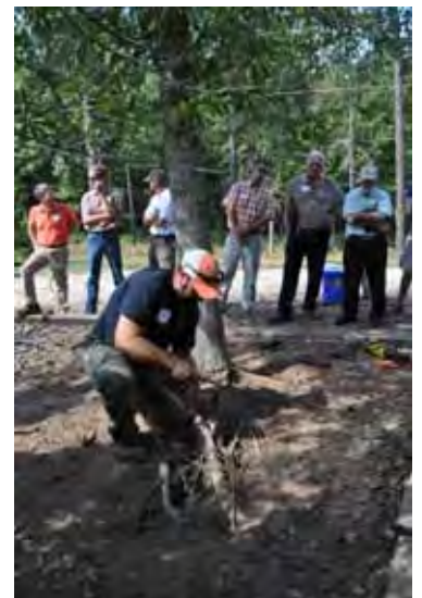
Nathan Dubosh (MUSC) explains the uses of an air spade and demonstrates the advantages over mechanical equipment.
