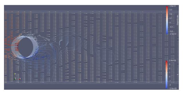
Figure C.5: Simulated flow behind a cylinder with 150mm diameter at 0.5m/s, with glyphs showing the flow velocities and contour lines showing the different pressure levels.
