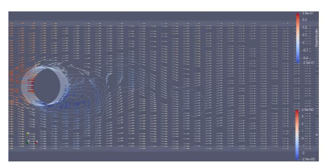
Figure C.6: Simulated flow behind a cylinder with 150mm diameter at 0.5m/s, with glyphs showing the flow velocities and contour lines showing the different pressure levels.
