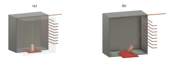
Figure D.1: Preliminary CAD design showing (a) an enclosure containing an elastic and conductive haircell and bearing strips of wiring embedded in one wall and (b) the haircell deflecting in response to a flow stimuli affecting its other end (not pictured) and being pressed against the strips of wiring. This action then complets the circuit and allows resistance to be measured, with that being dependent on how many strips of wiring in the wall the haircell crosses.
