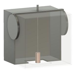
Figure D.2: Preliminary CAD design showing an enclosure containing a haircell made from a magnetic material positioned between two magnetic field sensors. As the haircell deflects in response to flows affecting its other end (not pictured), the magnetic field sensors detect and measure this.
