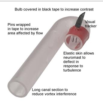
Figure 5.12: 3D printed physical sensor, with the elastic skin (red), artificial neuromast, and corresponding visual tracker (black).
