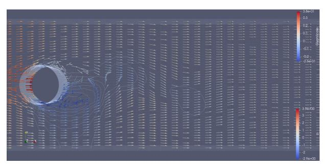
Figure C.4: Simulated flow behind a cylinder with 150 mm diameter at 0.5 m/s, with glyphs showing the flow velocities and contour lines showing the different pressure levels.
