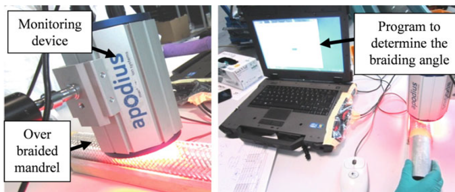
Figure 4.3: Apodius Vision System (AVS) used by Reimer et al. for braid angle and cover factor measurements; reproduced from [246].
