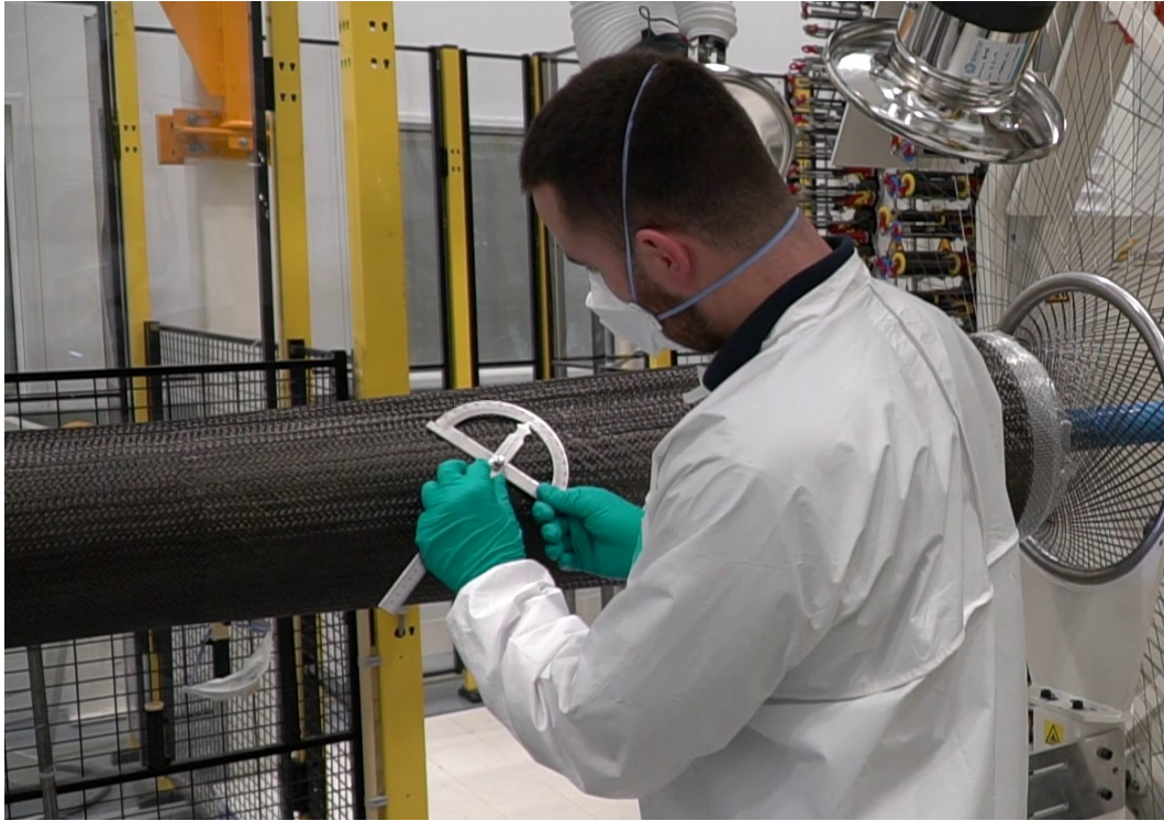
Figure 4.7: Manual measurement of braid angle is typically performed by the operator using a protractor.
