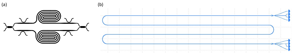
Figure 5.7: (a) Simplified schematic of the final devices. MZI with mode multiplexing and demultiplexing in each arm. Only one arm will be used, the other mode converters are included to balance loss. (b) Final design which was fabricated. Full etched silicon nitride device with grating couplers.
