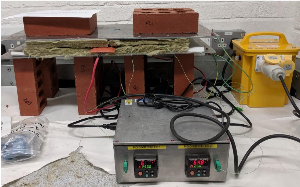
Figure 4.1: Photograph of heater mat apparatus, showing platform, aluminium plates, thermal insulation and heater mats (orange, protruding slightly from insulation material), feedback thermocouples and controller unit.
