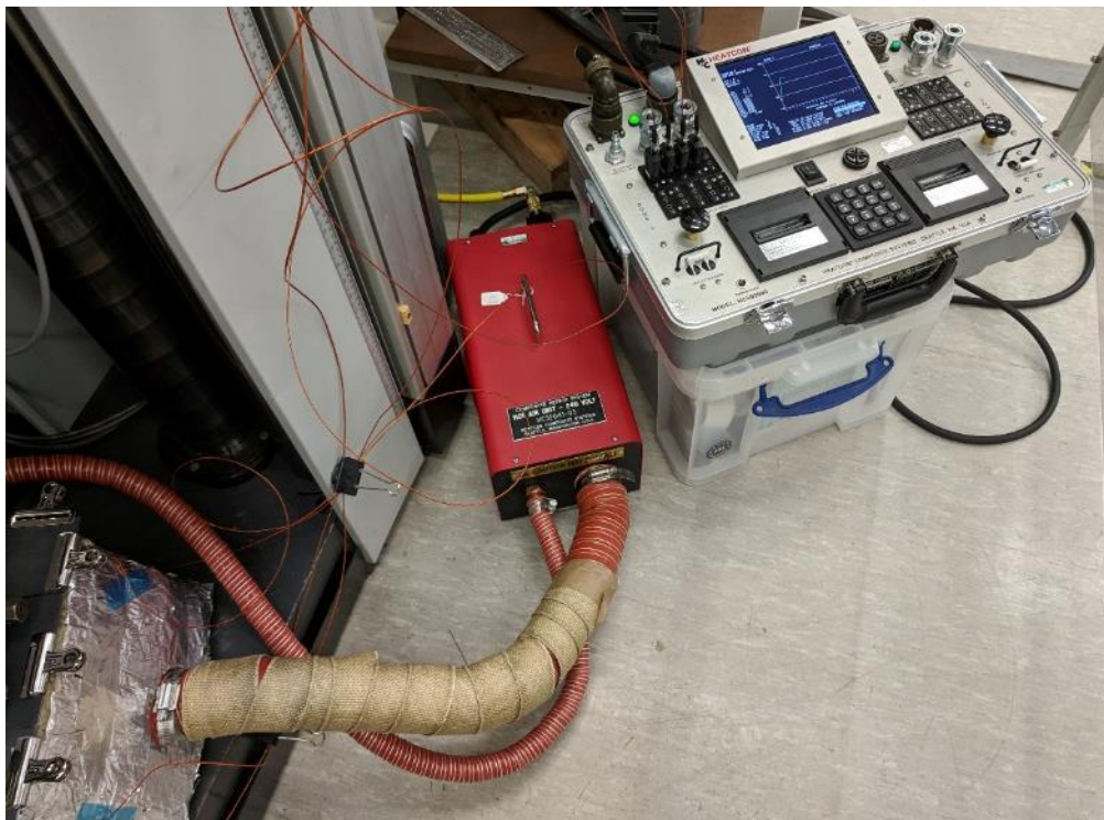
Figure 3.9: Photo of the Heatcon hot bonder and hot air curing systems connected to the thermal chamber.
