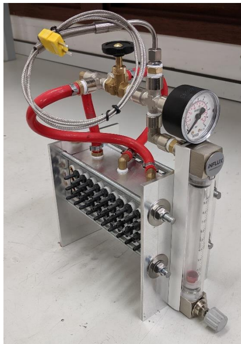
Figure 4.2: Photograph of coolant supply manifold, with flowmeter, control valves, pressure gauge and thermocouple visible.
