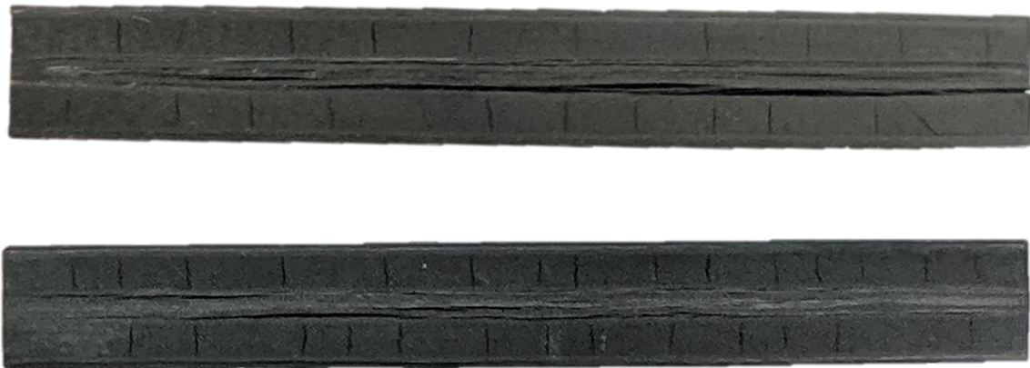
Figure 4.4: Photographs of the ends of an NV120 specimen, showing the intra- and inter-laminar cracks present.
