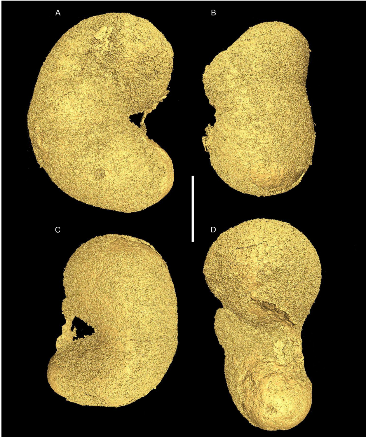
Figure 3.7. Isosurfaces showing morphotype 3 external morphology. (A-D) 3D surface renderings of the specimen ZY1216_11 from different view angles. Scale bars are 500 \mu\text{m} .
