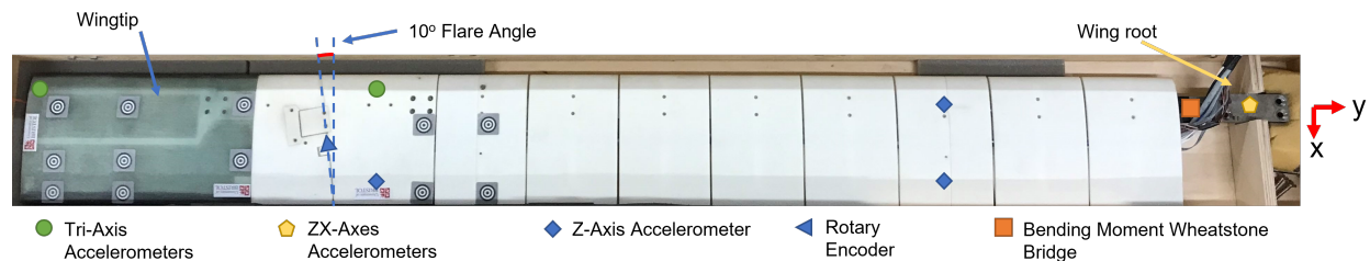
Fig. 7 An overview of the flexible semi-span model
