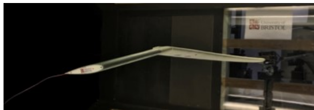
Fig. 8 The wind tunnel model coasting at a stable equilibrium position
