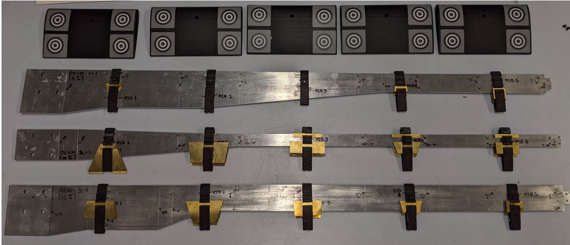
Fig. 13 Assembled wing spars with attached ribs and masses.
