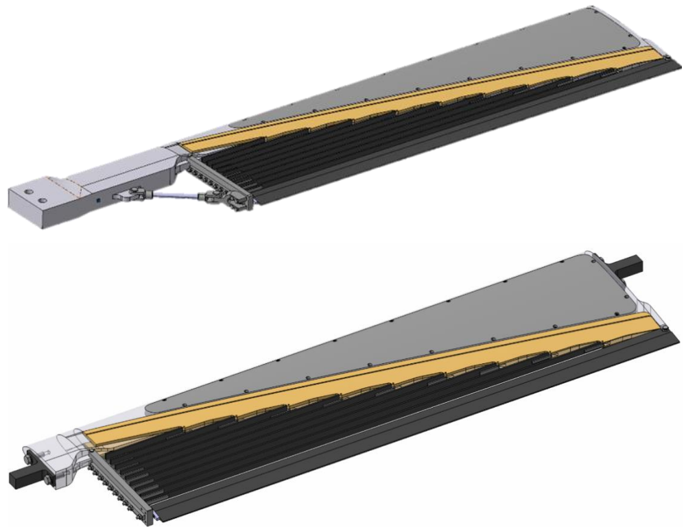
Figure 3. Modified demonstrator design with GFRP auxiliary spar for attachment of the elastic skin.
