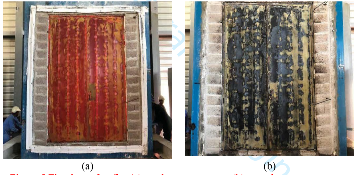
Figure 5 Fire door after fire (a) pre-hose stream test (b) post-hose stream test
