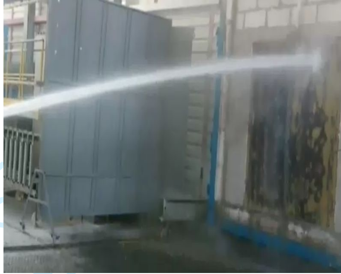
Figure 6 hose stream random jet cooling for the exposed surface under 4 bar water pressure
