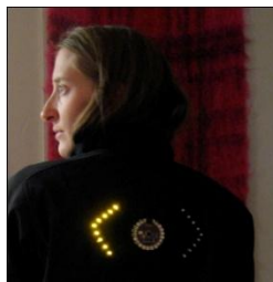
Figure 5: Proposed Jacket implementation of turn signals
