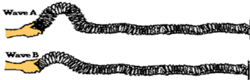
Figure 5.3 Slinkies A and B are Attached to the wall and Pulsed at Different Amplitudes
