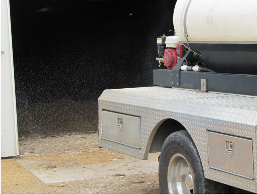
Fig. 2.8. Chemical sprayer truck applying insecticide inside a poultry house. (photograph by J. Talley)
