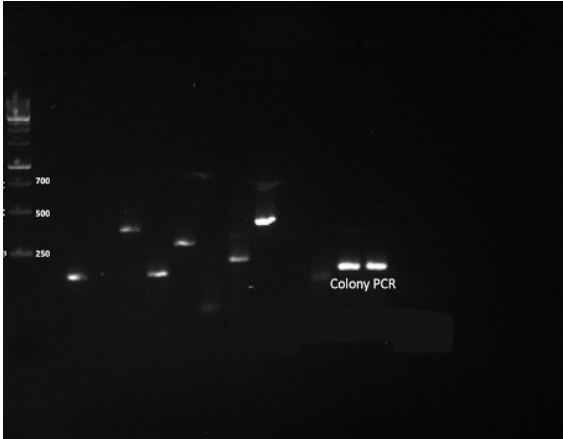
Fig. 3.3. Colony PCR gel electrophoresis. Colony PCR bands indicate primers amplified bacterial DNA that was approximately 163bp. Lane 1-1kb maker, lanes 2-10 unrelated samples, lanes 11-12 Enterococcus. cecorum colonies.
