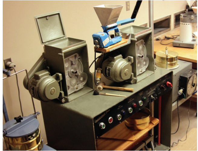
Figure 3. Brabender Quadrumat Senior Mill (modified shaker system).
