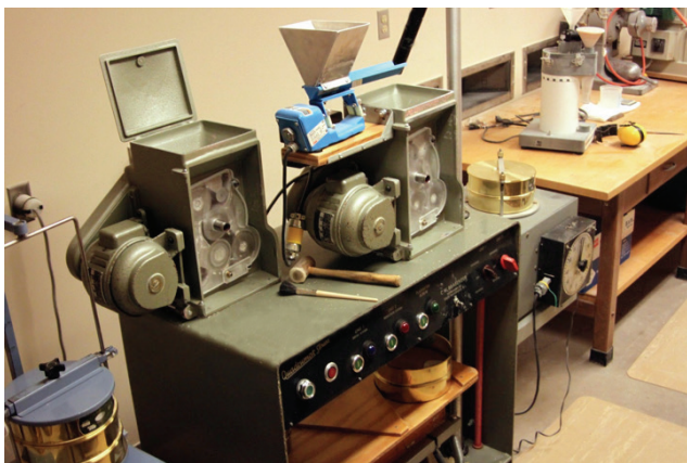
Figure 3. Brabender Quadrumat Senior Mill (modified shaker system).
