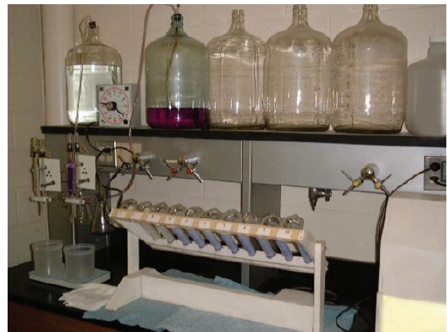
Figure 6. A sedimentation test is used to determine the quantity and quality of gluten.
