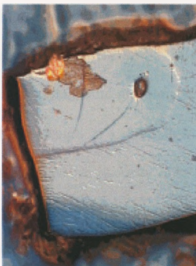
Figure 4.5: Larger samples of \text{Y}_2\text{O}_3\text{-Al}_2\text{O}_3 glasses formed by high- T melting in a Xe lamp thermal imaging furnace, and quenched by passing the molten droplets through a Pt wire grid. Here, the polished sample shows coexisting low density area (LDA) (top left) and the high density areas (HDA) matrix regions. The glassy polymorphs have different mechanical properties, resulting in a higher quality of polish for the LDA sample (from McMillan et al., 2007)
