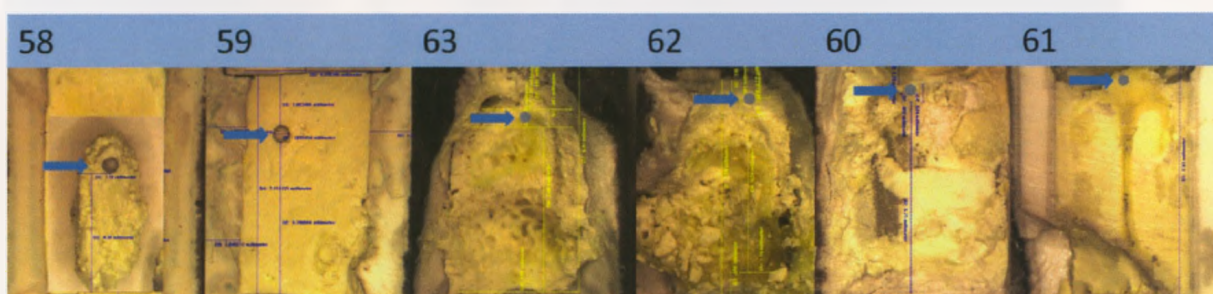
Figure 3.2: Sectioned and ground cubes showing sphere positions for experiments performed in the L' region (4.5 GPa, 1100°C). Numbers correspond to experiment numbers.
