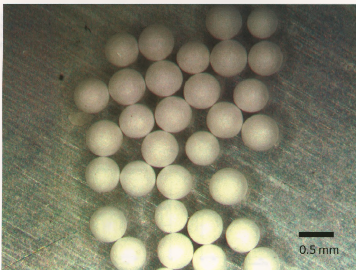
Figure A1.2: Photograph showing fabricated BN spheres shown for size uniformity.
