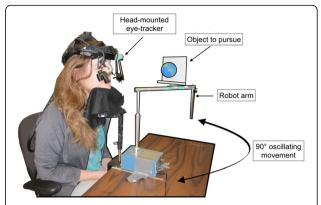
**Fig. 1** Experimental setup including eye-tracker, robot arm, and object to be pursued
