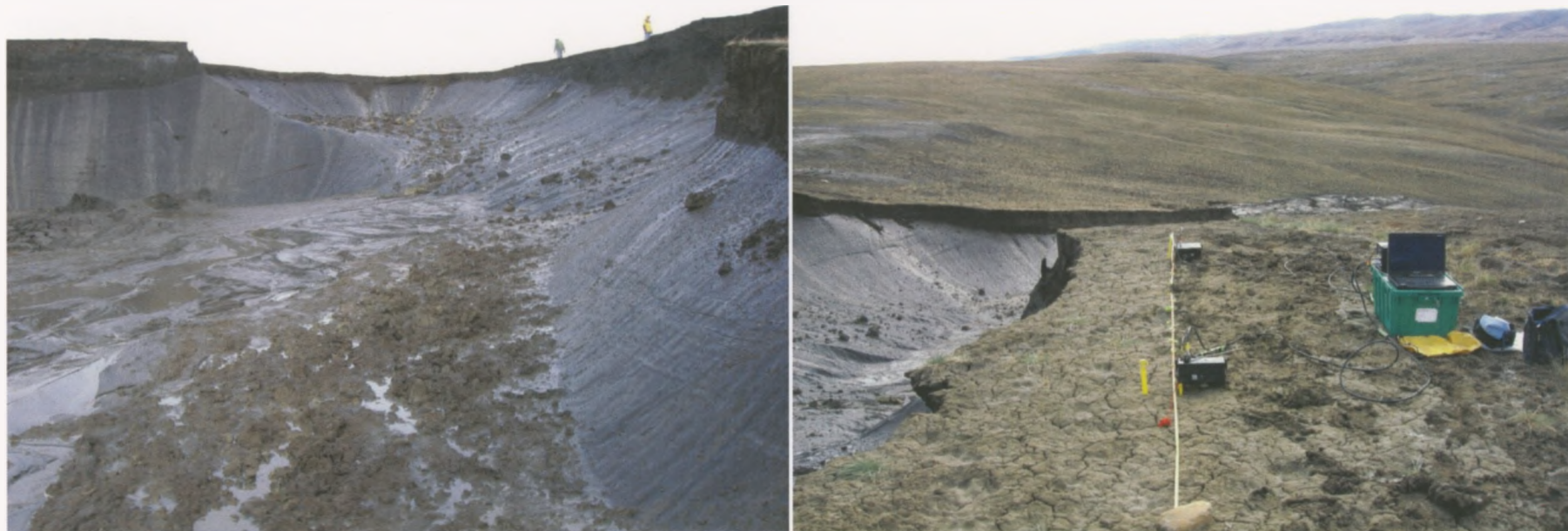
Figure A1-3. Right: Slump feature south of Slidre Fiord, Ellesmere Island with several metres of exposed stratified segregation ice. Left: Location of overburden surveys at the site. This transect line was then excavated for on-ice surveys.
