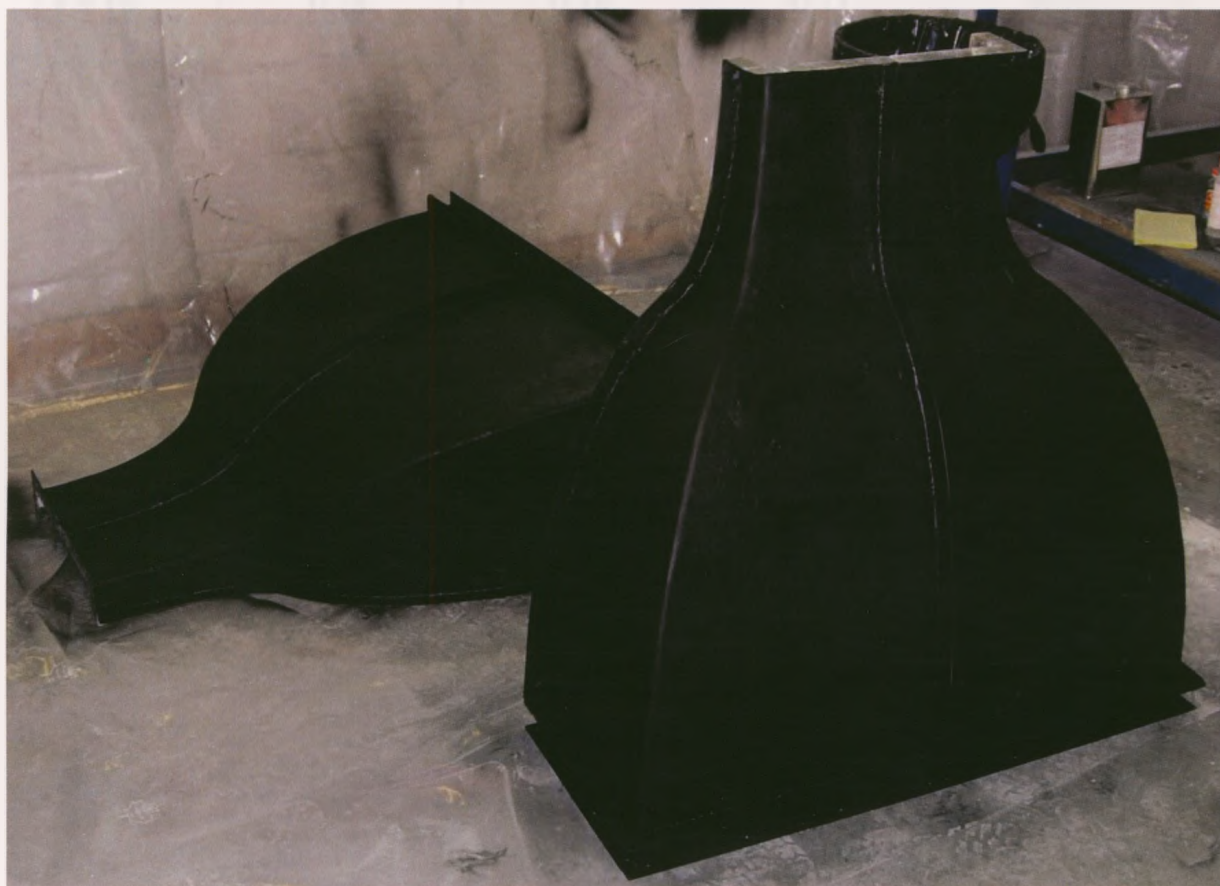
Figure 121: Finished fiberglass halves of inlet cone
