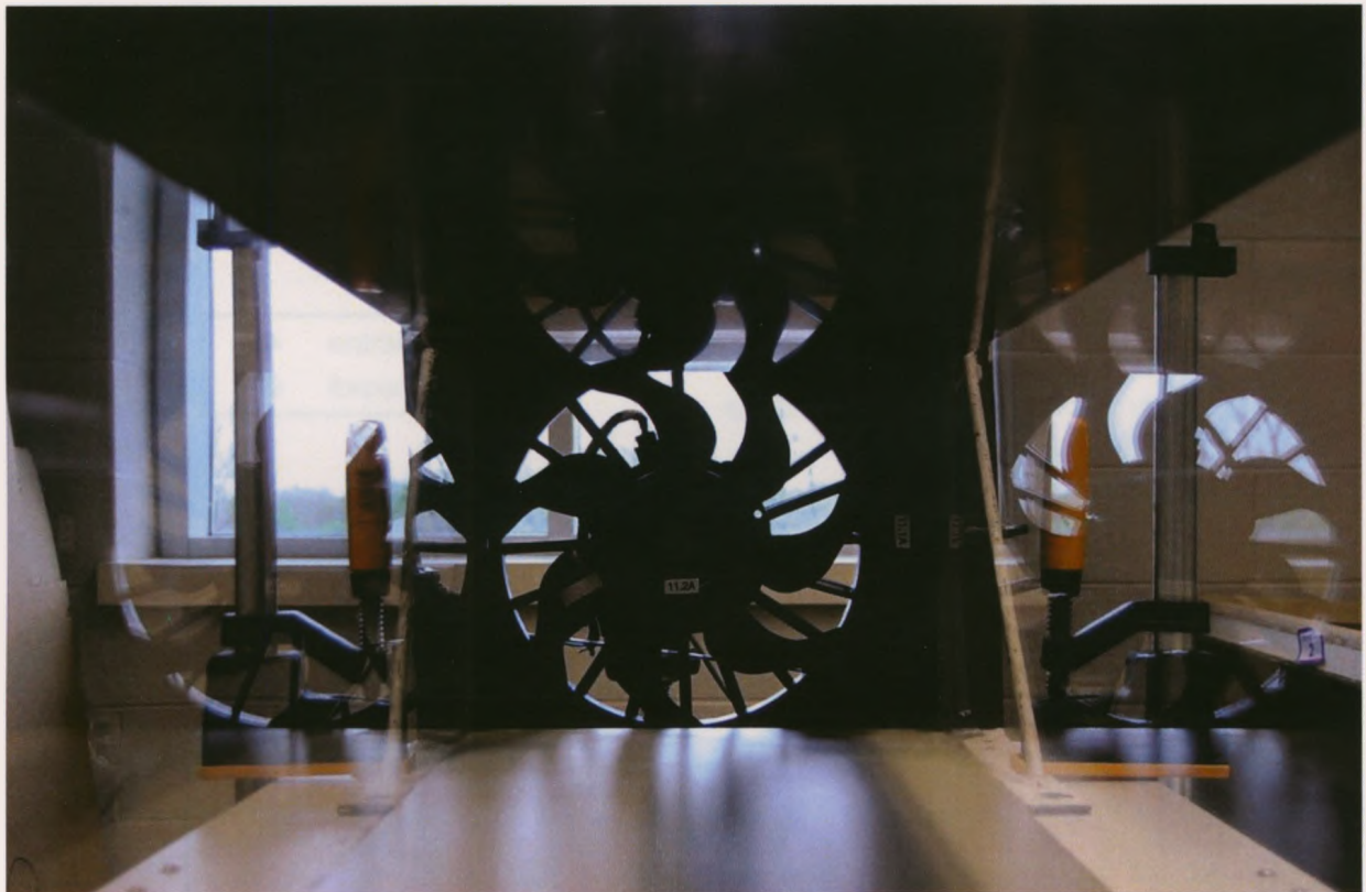
Figure 54: Automotive cooling fan mounted at exit of wall jet tunnel to force a co-flow
