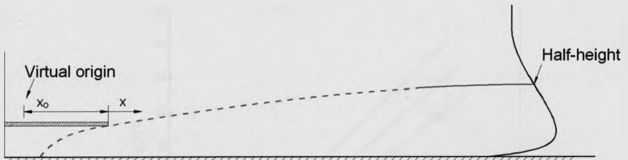
Figure 3: Example of using a superficial origin. (Dashed in red) A wall jet would be developing and the dashed half-height curve is not realistic but a result of the formulae. (Solid in red) A wall jet profile has developed.
