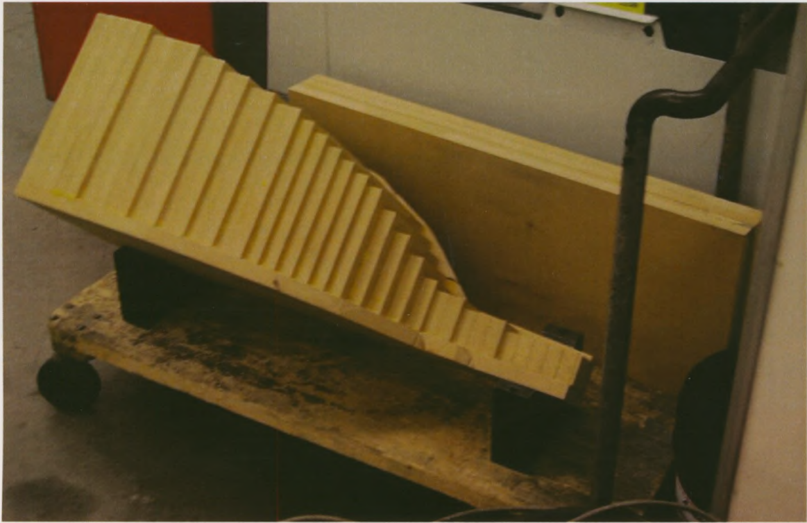
Figure 118: High-density fiber board stacked to roughly shape the inlet cone mould
