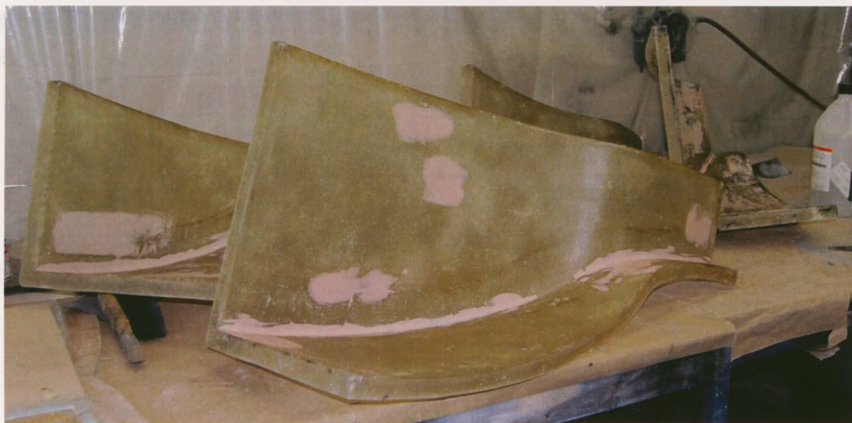
Figure 120: Fiberglass portions of the inlet cone with imperfections smoothed with automotive body filler
