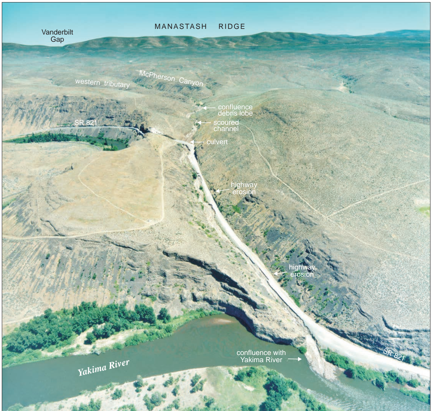
Figure 7. Looking northeast from the mouth of McPherson Canyon to the summit of Manastash Ridge. Note the scoured channel between the highway crossing of McPherson Canyon and the confluence debris lobe. Erosion from the overflow of the culvert can be seen paralleling the highway downstream to the Yakima River. The catchment area for the debris flow in McPherson Canyon lies beyond the left side of the photo (Fig. 4). Photo courtesy of the Washington State Department of Transportation.
