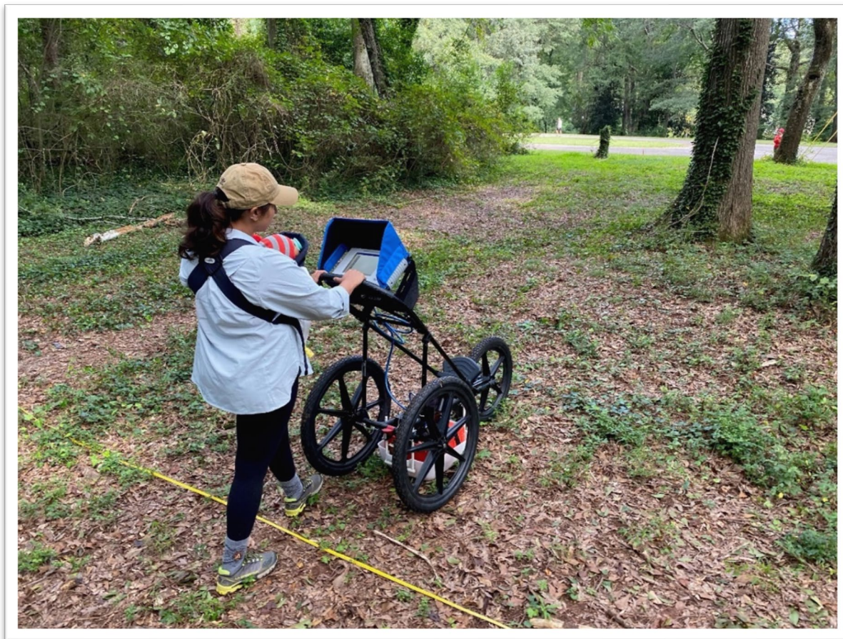
Figure 4.1 A Photograph of GSU's SIR-3000 GPR being utilized to survey a grid at the Farmer Street Cemetery
