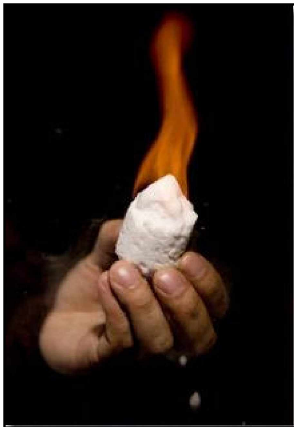
Figure 2.1: Burning Sample of Methane Hydrate (Courtesy National Research Council, Canada, Website: www.nrc-cnrc.gc.ca )
