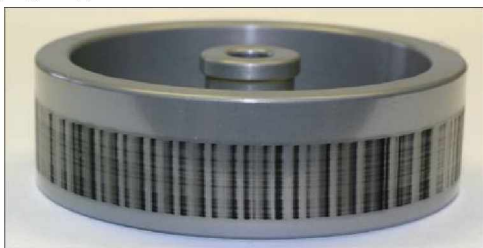
Figure 2: Drum. Side view of a cylindrical drum from a DRUM impactor.
