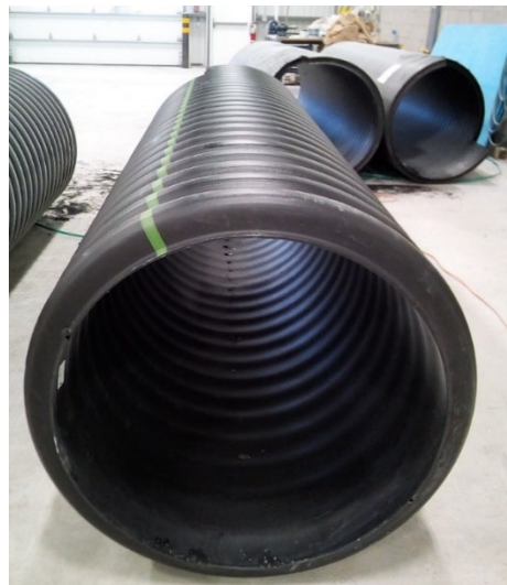
Figure 2.1 HDPE pipes under investigation
