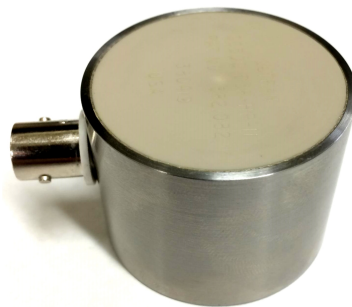
Figure 4.5 Example of a 50.8 mm diameter Ultratran transducer
