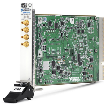
Figure 4.9 PXI-5412 waveform generators (from NI website)
