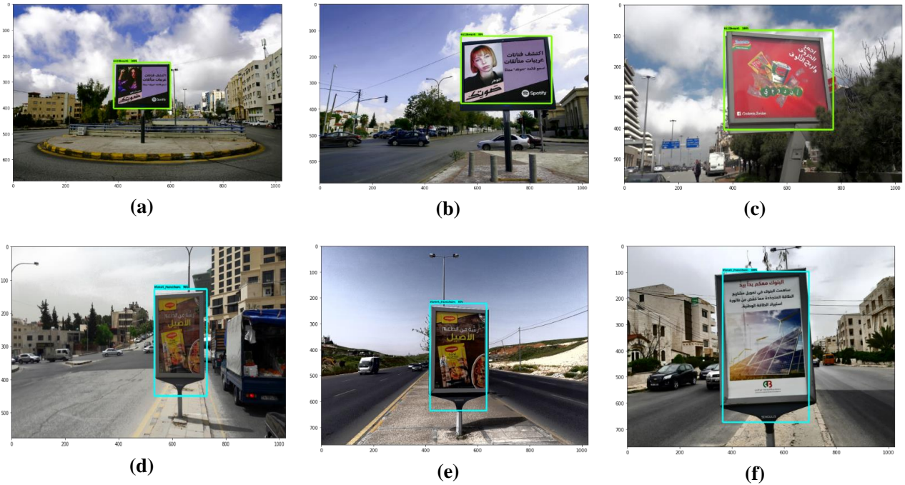
Figure 5. Examples of the final network performance in detecting the two classes of billboards using unseen testing images: (a)-(c) Roadside Billboards; (d)-(f) Street Furniture Billboards
