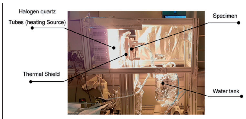
Figure 1. Developed test apparatus. 18
