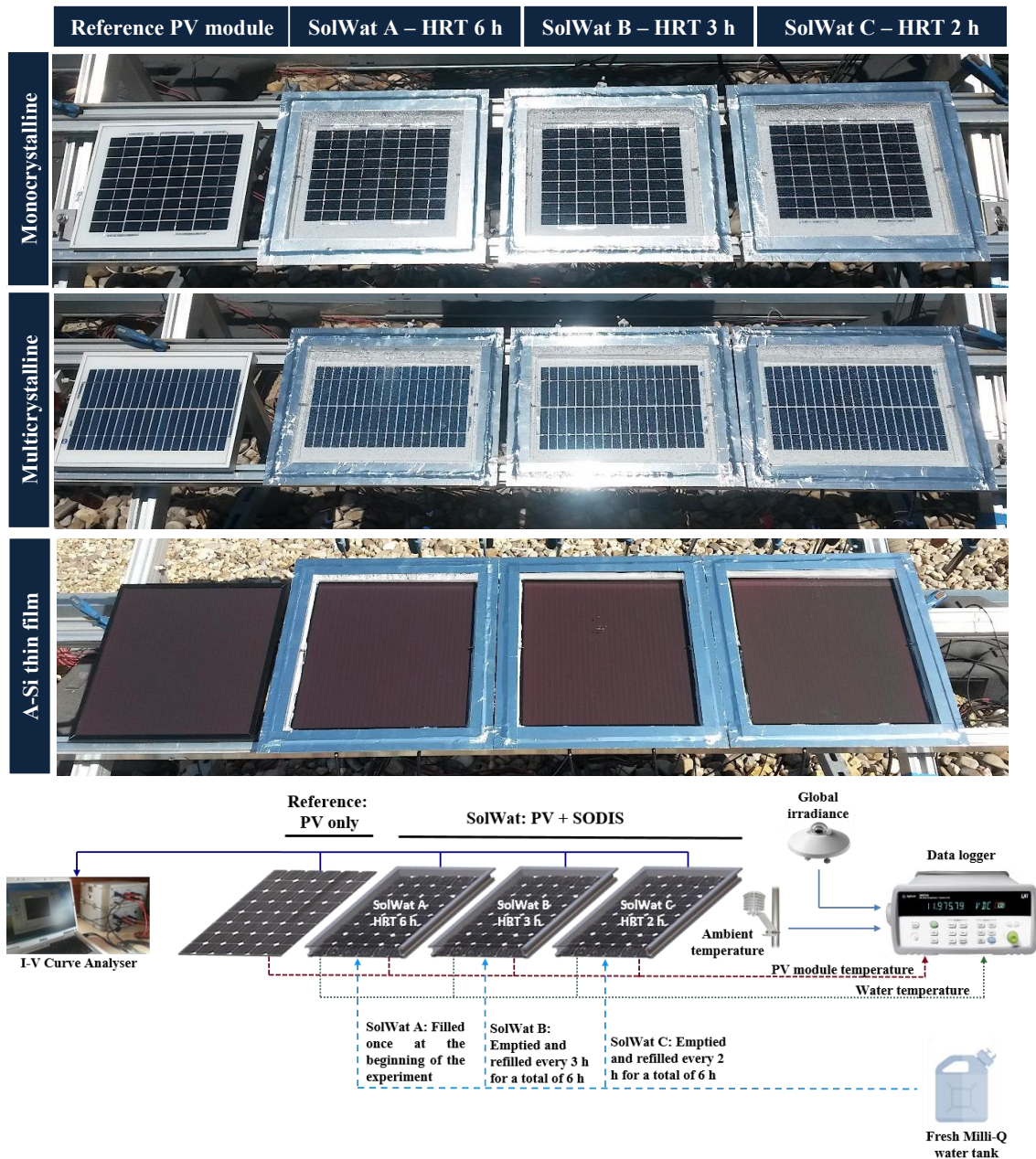
Figure 2. Reference panels and SolWat systems of monocrystalline, multicrystalline and a-Si thin film technologies to assess the effect of the water disinfection reactor on top of the PV module at different hydraulic retention times (6, 3 and 2 hours). Each experiment was composed by three SolWat systems and a reference panel (without the water chamber on top) of the same PV technology and characteristics. It is included the schematic diagram of data acquisition and recording system including the flow chart of the hydraulic retention and the reactors layout.
