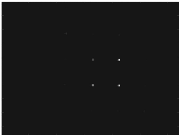
FIGURE 8 Intensity image captured by the QuantiCam SPAD array, for projection of a 2 \times 2 grid of spots
