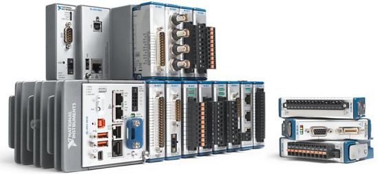
Fig. 7. Image of NI cRIO Chassis populated with C-series DAQ modules. [14]
