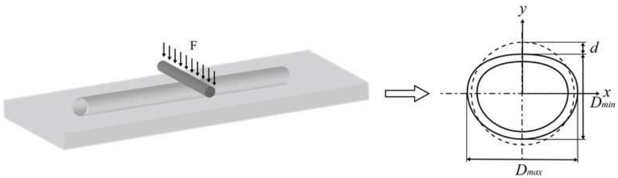
Fig. 17. Schematic of two types of deformation manufacturing processes.
