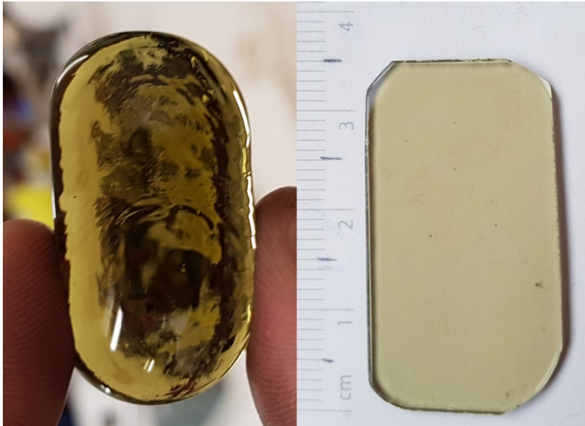
293 Figure 5 Transparent glass made from regolith simulant LHT-3M. Sample after casting and annealing (left) and after 294 processing (right).
