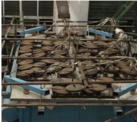
(a) Photos of the iron bricks and restrained beams at each corner
