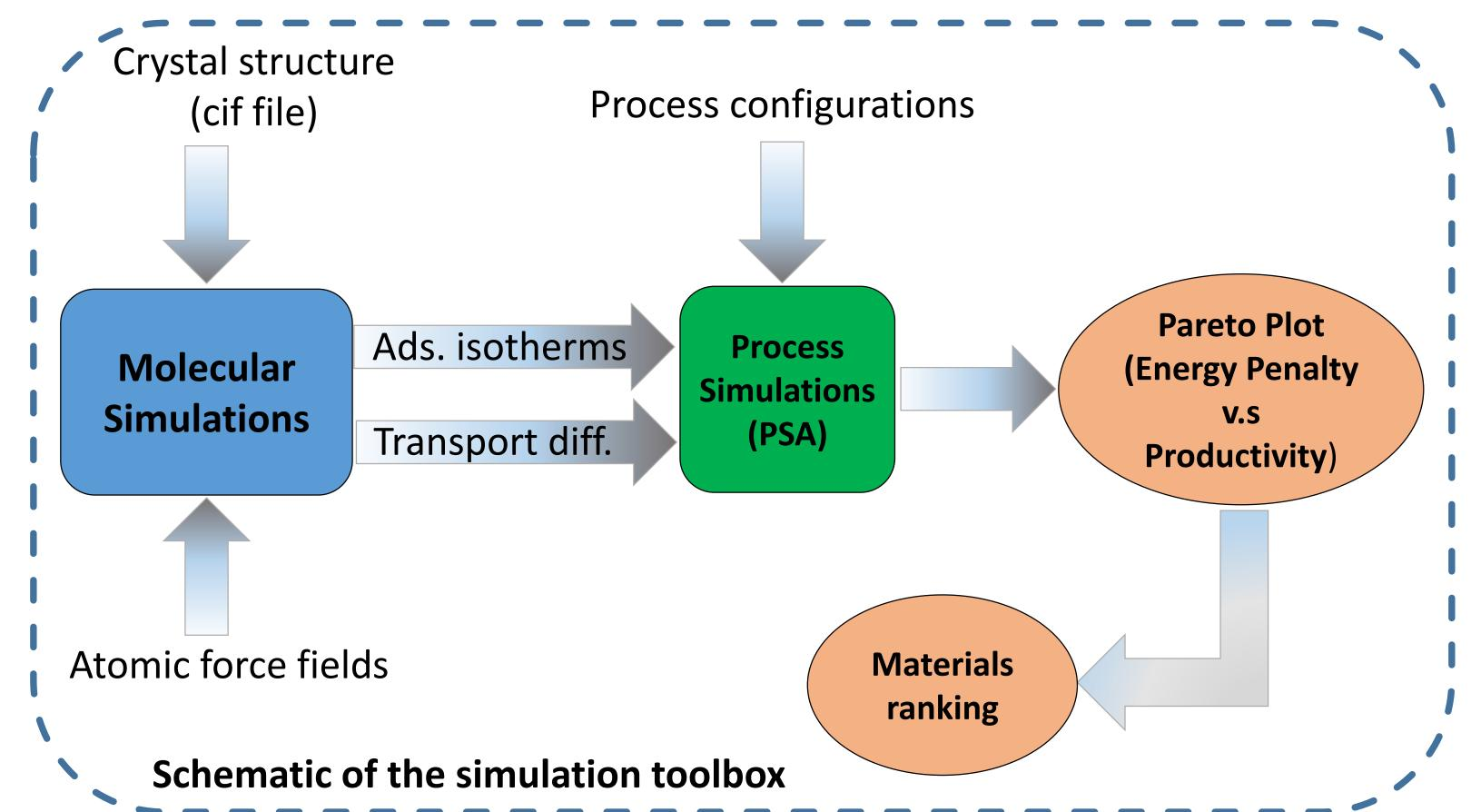
• A process modelling and optimization toolbox is under development in which molecular simulations provide equilibrium and transport data, while the materials ranking is performed in the process scale where effects of process configuration, materials stability and process cycle parameters are taken into account.
