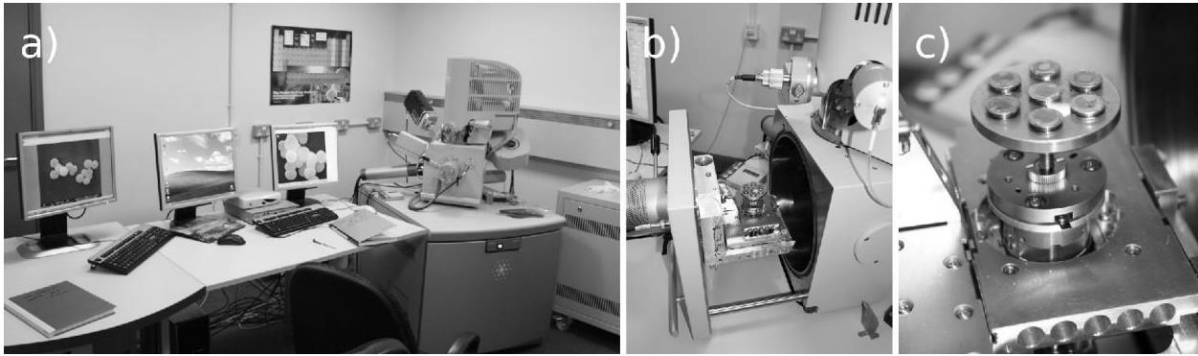
Figure 3.9 Images of FEI Inspect F scanning electron microscope. a) microscope general view, b) vacuum chamber with specimens fitted, c) sample holder with specimen close-up.
