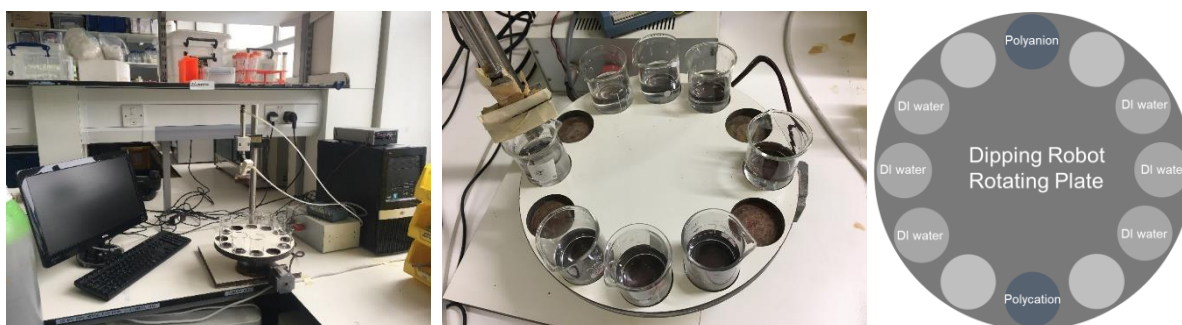
Figure 3.4 Images of homemade Layer-by-layer dip-coating machine. a) the general view of the dipping robot. b) the rotating plate and dipping pole while running. c) the polyelectrolyte solution and the DI water beaker positions on the dipping robot rotating plate.
