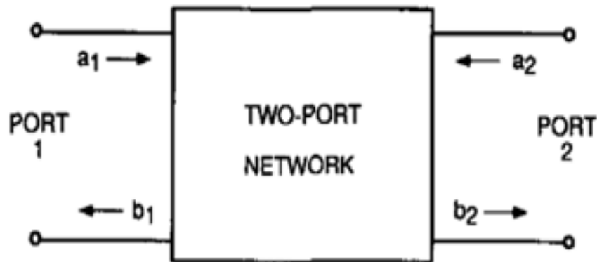
Figure 59 The general view of two-ported system with ABSD parameters defined(here they are a_1 , b_1 , a_2 and b_2 ).
