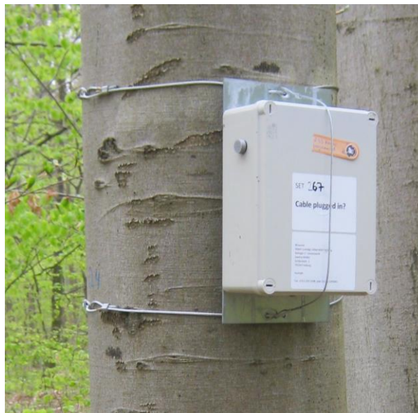
Figure 4.2. A Luniletronik Soundscape Explorer device attached to a tree in Hainich National Park, Germany.
