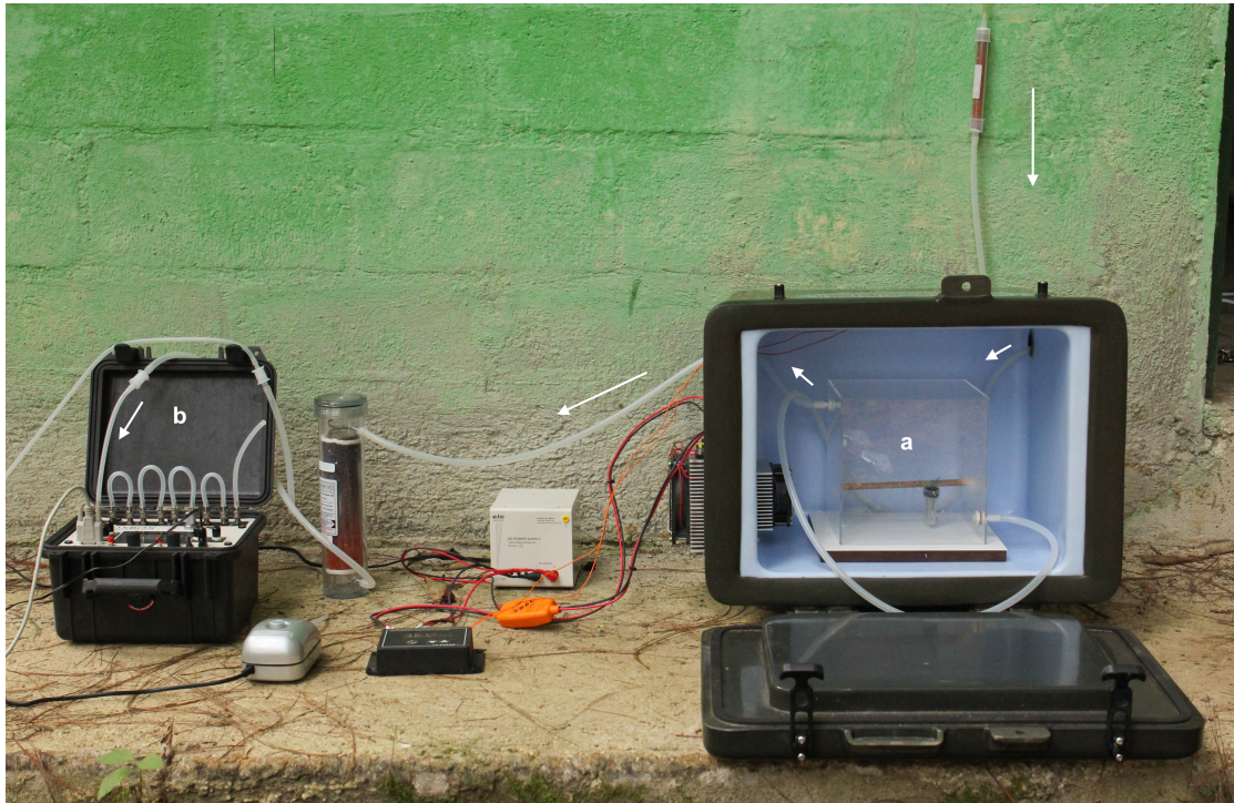
Figure 1.2 Field respirometry system used during this study. White arrows display the direction of airflow pulled through the chamber (a), in which a bird is placed and to the gas analysers (b; FoxBox, Sable Systems, USA). The larger box surrounding (a) (when closed) manipulates temperature.
