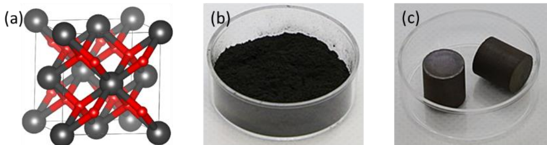
Figure 1.6: (a) Cubic structure of \text{UO}_2 ; (b) \text{UO}_2 powder; (c) \text{UO}_2 pellet. 3
