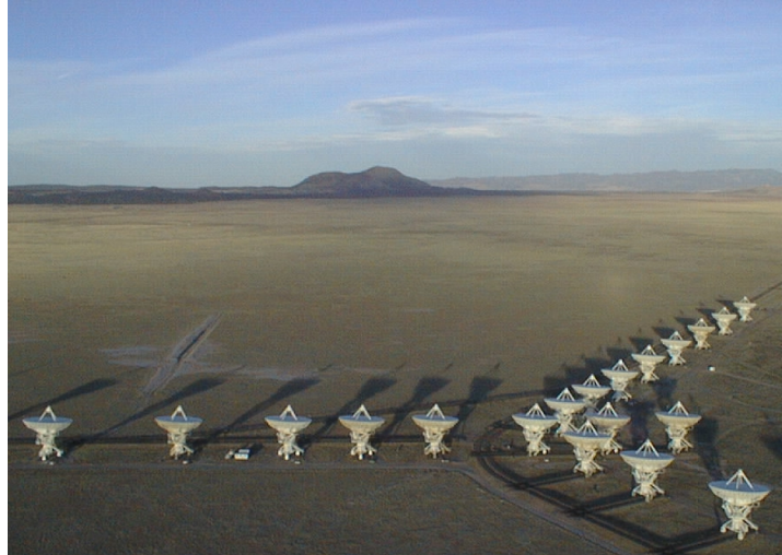
Figure 1.3: The Very Large Array, a radio telescope array which relies on the principle of interferometry. From nasa.gov
