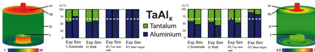
Figure 4.3: Measured composition at various points within a vacuum chamber for low pressure (2 mTorr Left) and high pressure (20 mTorr right) [148].
